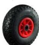
*The 831, 833 and 834 pneumatic wheel series are made without air inside, as they are filled with polyurethane foam (831 and 833) or are solid (834). This means that they can not suffer punctures or pressure losses.*
